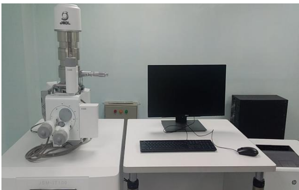
Figure 2: Scanning Electron microscope (JEOL, Tokyo, Japan, Model No. JSM-IT 100).
