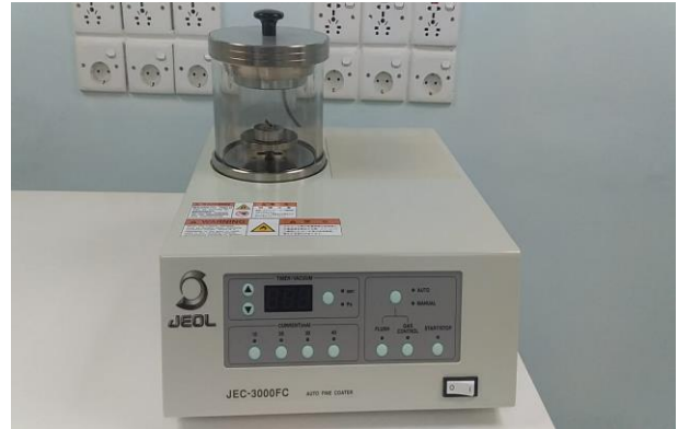
Figure 3: Metal stubs and titanium sputtered in the JEC-3000FC Auto Fine Coater.
